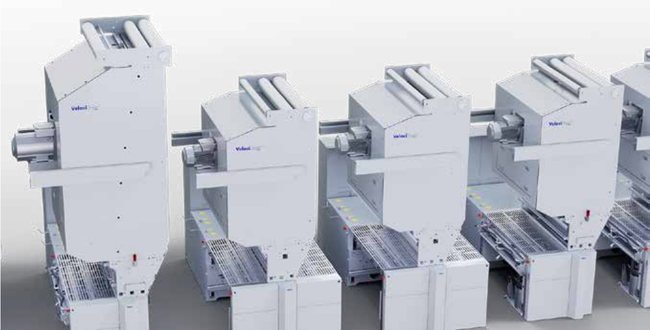
Modular design allows for any requested combination of Single- or Dual-ink-Deck units
